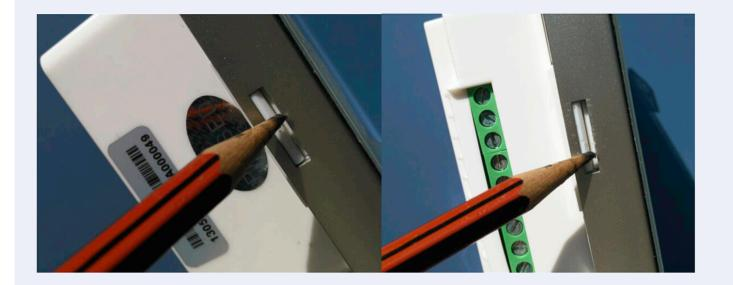
There are spring locks in the two sides of the Wall Control. Push both the spring locks slightly, then take the main part out to separate the back cover and the main part. You will see the PROGRAM/CODE button on the main part.
