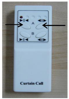
Press the "A" Open <u>or</u> Close button in turn back and forth 4 to 5 times, or till the Motor turns.
