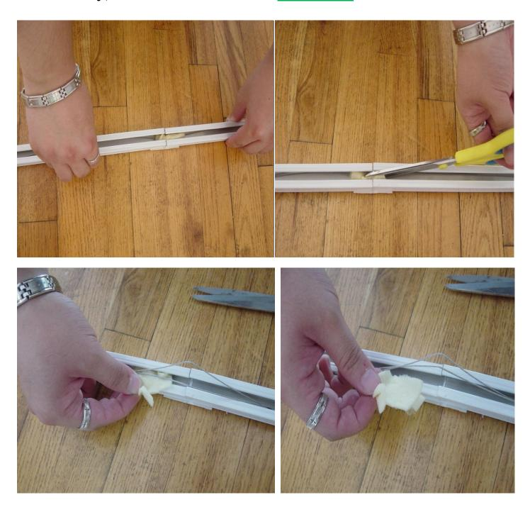
IV) Slide the <u>Track Connector</u> to the middle of the 2 <u>Tracks</u>. In the mean time, push the 2 <u>Tracks</u> toward each other as close as possible.
