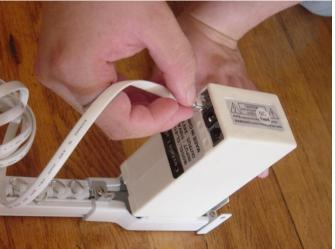
In case to remove the <u>Motor</u>, press down the 'knob', turn the <u>Motor</u> 45 degree either direction and pull it up at the same time. It should be out of the socket easily.
