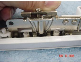
XI) Check if the <u>Steel Wire</u> is taut and adjust it by turning the <u>Hexagon Screw</u> at the end of the <u>Motor Socket</u>.
