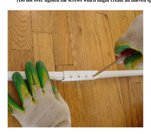
VI) Unscrew the top screw on <u>Carrier-A</u> and take out the <u>Metal</u> <u>Clip</u>. (Remember how the <u>Steel Wire</u> is placed as V-shaped)
