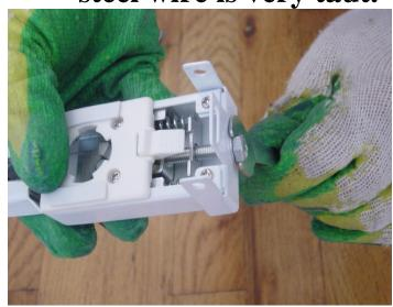
Check if the <u>Steel Wire</u> is taut enough by pushing it with something. It should not be bent by pushing it and it should be straight and taut. If not, turn the Hexagon Screw more to make sure it is taut.
