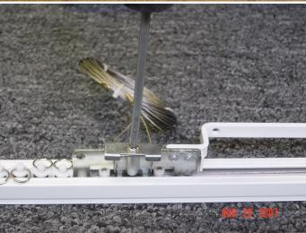
VI) Turn the Hexagon Screw to make sure the silver wire inside the track is straight and <u>taut</u>.
