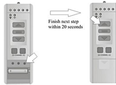
1.Press SET button for 5 seconds. then loose SET button when the sound changes from short whistle to long whistle. At this time, the motor will turn into the setting state.
