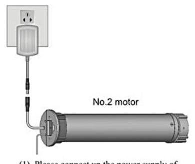
Please connect up the power supply of No.2 motor after 30 seconds when the No.1 motor's setting has finished.
