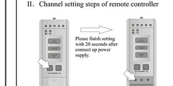
1. Press left/right channel button to turn channel 1 light on( or any channel that you like)
