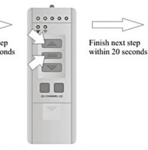
4. Press STOP button firstly, then press UP button at the same time. Loose two buttons when there sounds a long whistle, then upwards setting has been finished.
