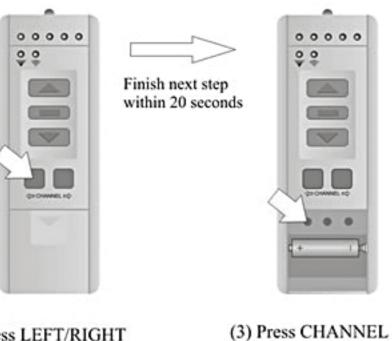
(2) Press LEFT/RIGHT CHANNEL buttons to turn channel 2 light on. (or other channel lights that you like) Set positions The setting steps are just the same as Step III.
