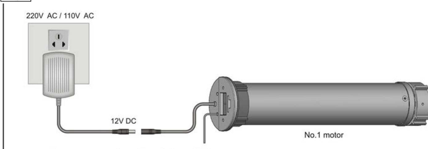
**Connect the power to the Motor, within 20 seconds, there will be a short whistle which means it is in programming mode.**
