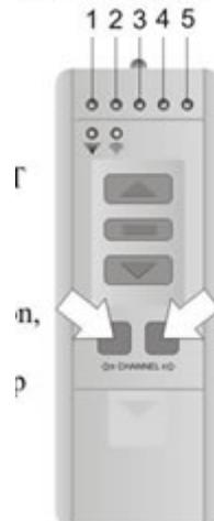
Press LEFT and RIGHT Channel buttons at the same time, all channel lights will be on. Press UP/DOWN button to operate all systems.
