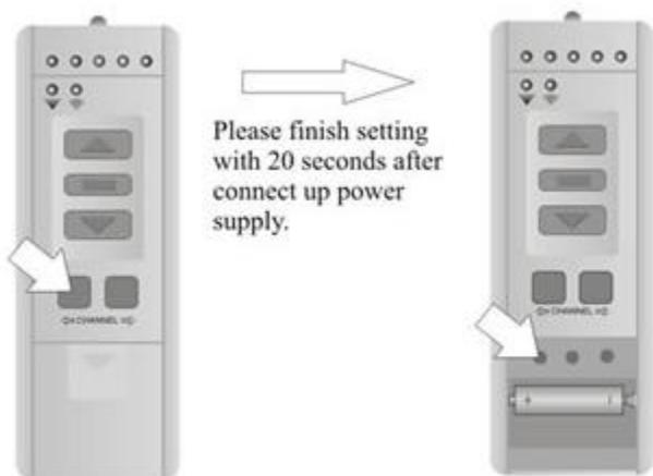
Press left/right **Channel** button to turn channel# 1 light on (or any channel number that you like)
